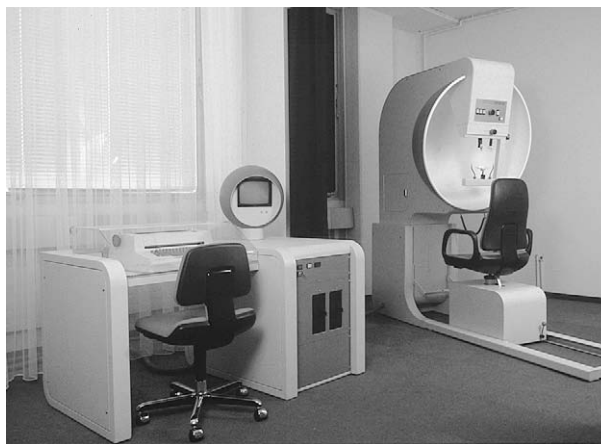
Fig. 3. The first commercially available fully automated perimeter to determine differential light sensitivity threshold, the Octopus 201. The instrument needed a lot of space.
